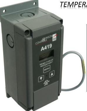
The A419 electronic temperature control is a single-stage, single-pole double-throw (SPDT), electronic temperature control. The control features a lockable, three button touchpad for setup and adjustment and an LCD which displays the sensed temperature and other control functions. A front panel LED indicates the output relay status. The control has a temperature range of - 30°F to 212°F.
