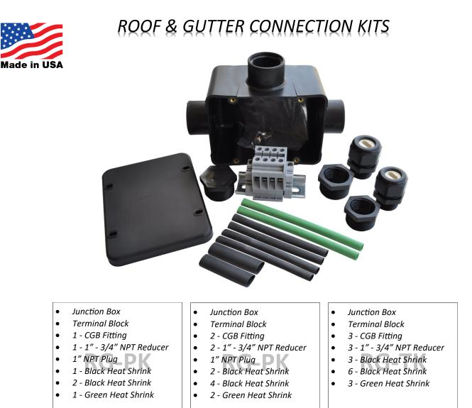
The SCK-2 power termination kit is for terminating self-regulating or constant wattage heater cables into a NEMA 4X enclosure (customer supplied) through a CGB fitting. The kit comes with heat shrink tubing to isolate each conductor including the ground braid. The SCK-2 is ideal for use in roof and gutter applications and comes with wire nuts for connecting to service leads.
